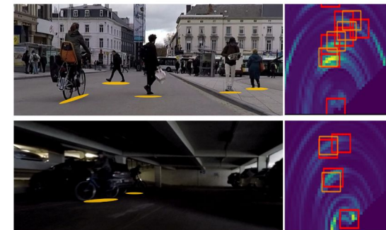
Fig. 1. An example of the radar scan and the synchronized camera image in different light condition. Orange and red bounding boxes represent the ground truth targets and results predicted by our proposed method. The radar scans have been visualized in Cartesian coordinates for comparison with the images.
